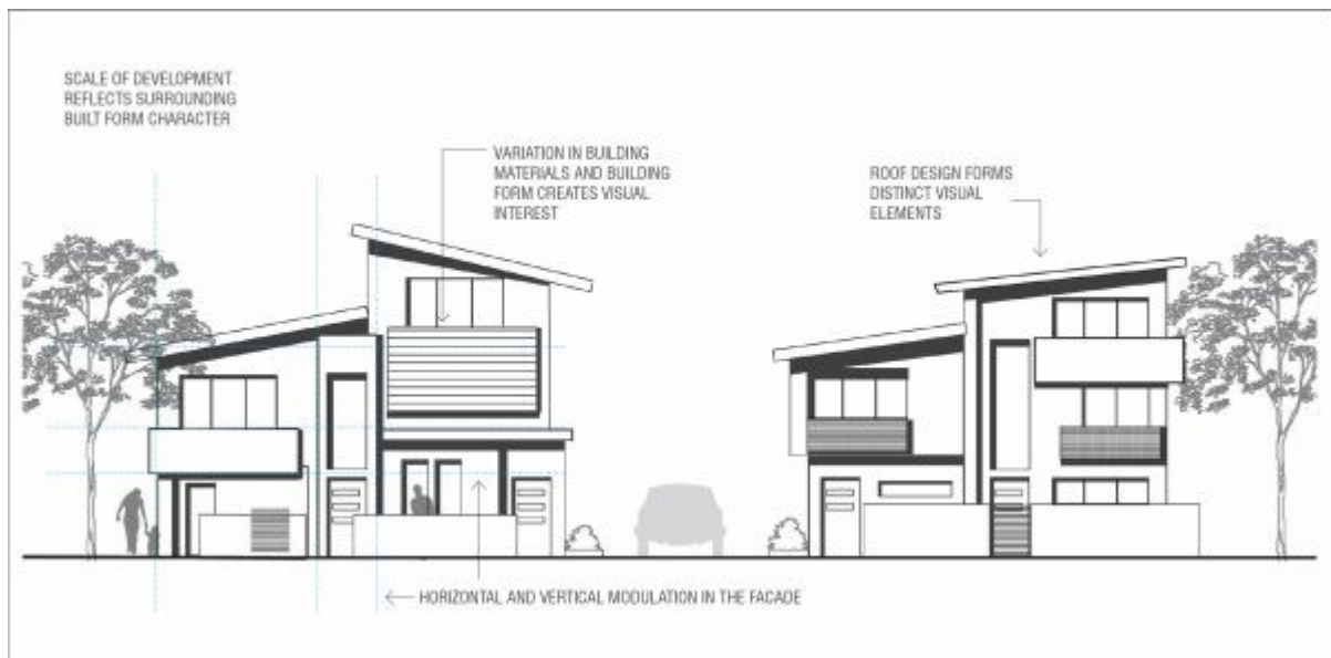
Figure 6.7 Building design elements
