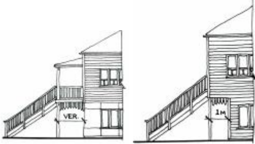
Figure 6.70 — Appropriate enclosures to the ground floor
